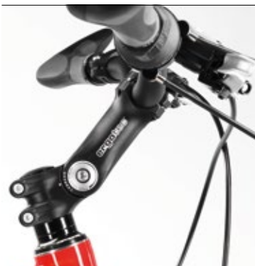
Stem with adjustable angle!
