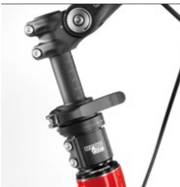
Stem with adjustable angle!
